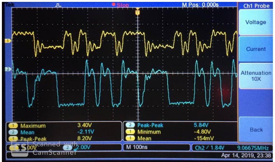
Figure 17: Final Result after comparator at 35MHz clock and 10m long POF
